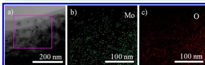
**Figure 4.** (a) STEM image of AA reducing MoO<sub>3-x</sub> nanodots (molar ratio of AA:Mo = 8); (b) STEM EDX mapping of Mo and (c) O signals.
