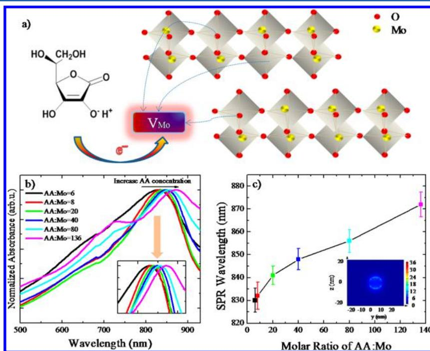
**Figure 5.** (a) Schematic diagram of AA reduction process for MoO<sub>3-x</sub> defects. (b) UV–vis absorption spectra of MoO<sub>3-x</sub> nanodots aqueous with various AA doses. (c) The corresponding response of oxide SPR peaks as a function of molar ratio of AA reductant/Mo source.
