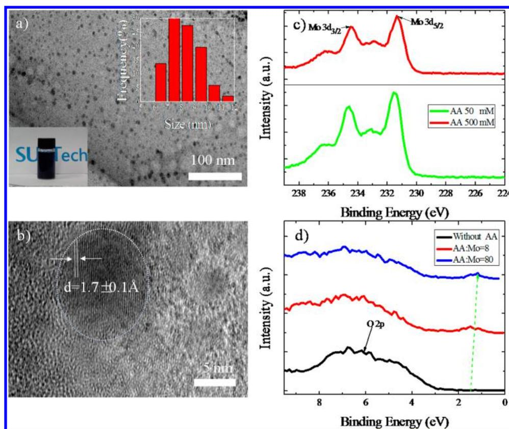
**Figure 3.** (a) TEM image of  $\text{MoO}_{3-x}$  nanodots with AA reduction (molar ratio of AA:Mo = 8). Inset: photograph of  $\text{MoO}_{3-x}$  solution. (b) HRTEM image for  $\text{MoO}_{3-x}$  nanodots with the same sample. Inset: SAED pattern of  $\text{MoO}_{3-x}$  nanodots. (c) XPS spectra of Mo 3d and (d) O 2p of  $\text{MoO}_{3-x}$  with 8 and 80 molar ratio AA reduction.
