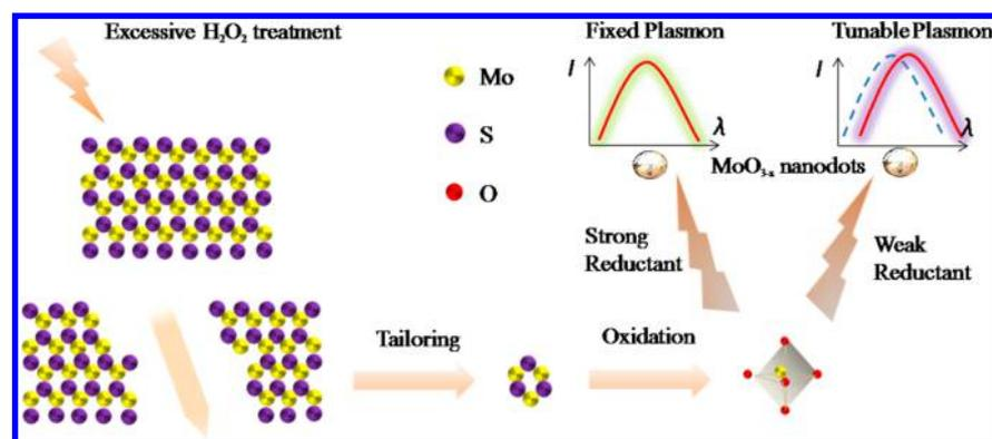
**Figure 1.** Schematic procedures demonstrate the  $\text{MoO}_{3-x}$  nanodots prepared from  $\text{MoS}_2$  nanosheets during oxidation and reduction process.
