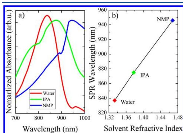
**Figure 6.** (a) SPR response of MoO<sub>3-x</sub> nanodots in different solvents. (b) Observed SPR wavelength as a function of the refractive index of the solvents.
