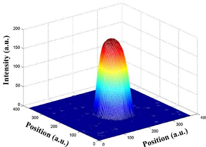
Fig. 5. The three-dimensional intensity distribution of the focal point.
