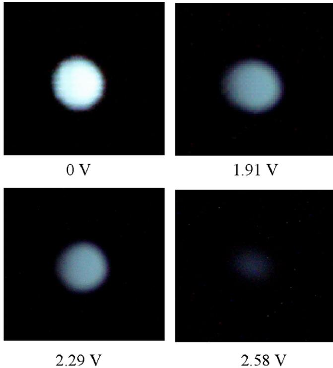
Fig. 4. The facula intensity at the focal point vs. different voltages applied. The applied voltages are 0, 1.91, 2.29, and 2.58  $V_{\text{rms}}$ , respectively.
