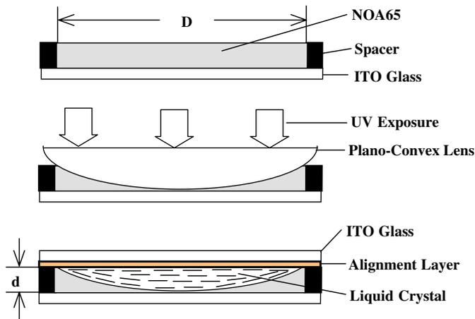
Fig. 1. The fabrication procedure of focus-switchable polymer-LC lenses,  $D$  is the diameter of spherical lens, and  $d$  is the center thickness of lens.
