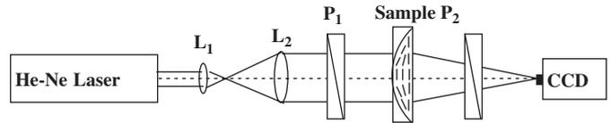
Fig. 2. Experimental setup to characterize the optical properties of the spherical lens.  $L_1$  and  $L_2$  are lenses to collimate the light beam.  $P_1$  and  $P_2$  are linear polarizers to control the polarization of light. A CCD is placed on the focus of the spherical polymer-LC lens to detect the facula.
