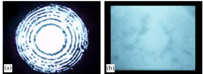
Fig. 3. The magnified interferogram pattern with no voltage applied. (a) and (b) show the magnified images obtained by CCD with no voltage applied when the rubbing direction of LC lens was orientated at  $45^\circ$  with respect to the fast axis of the linear polarizers and the rubbing direction was parallel to the polarizer's fast axis, respectively.
