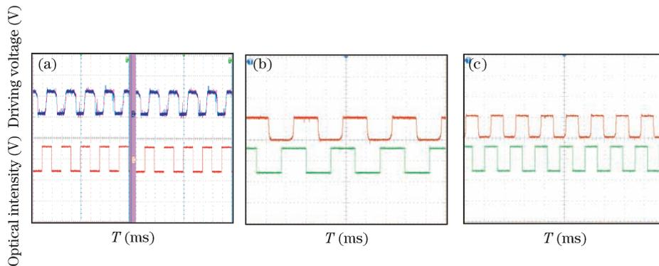
Fig. 5. Standard experimental curves of the mechanical optical chopper (a) 50 HZ, 10 ms/unit; (b) 100 HZ, 4 ms/unit; (c) 200 HZ, 4 ms/unit. Upper lines indicate the optical intensity curves, lower lines indicate the synchronous references.
