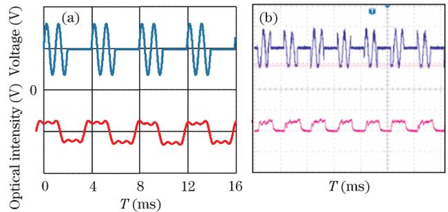
Fig. 3. (a) Simulation and (b) experimental results of the H-PDLC Chopper in generating a rectangular wave with 250 Hz.
