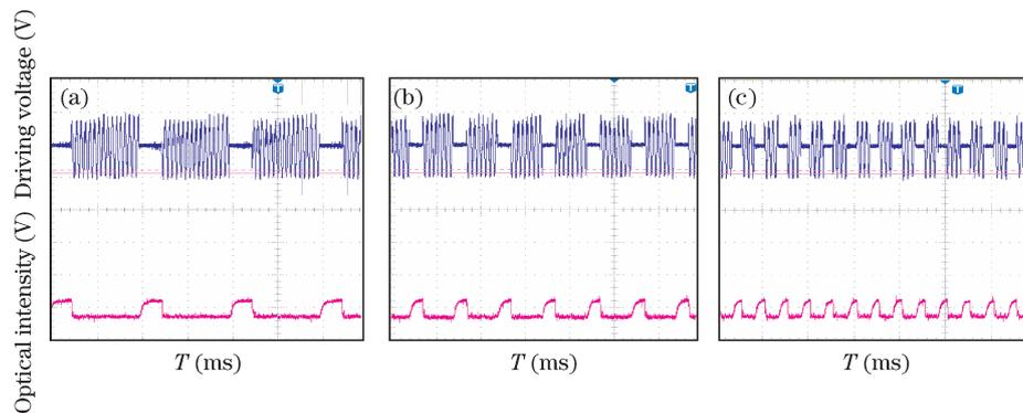
Fig. 6. H-PDLC chopper working with different duty cycles and frequencies: (a) 3:1 at 50 Hz, (b) 7:3 at 100 Hz, and (c) 3:2 at 200 Hz.
