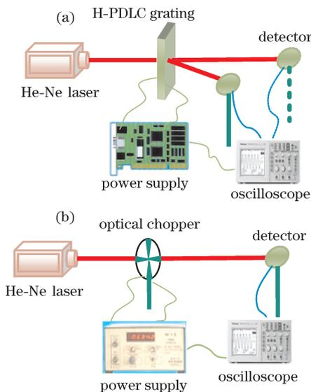
Fig. 2. Measurement setup for (a) the H-PDLC chopper and (b) the mechanical chopper.
