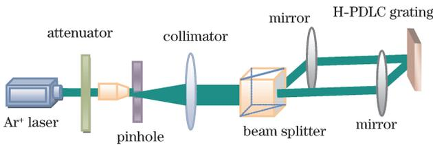
Fig. 1. Experimental setup used in fabricating the H-PDLC.
