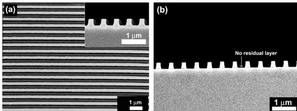
**Fig. 2.** SEM images of the first PMMA layer fabricated by reverse nanoimprinting (a) before and (b) after reactive ion etching. Inset of Fig. 2(a) shows the cross-sectional view of PMMA layer with  $\sim 80 \text{ nm}$  thick residual layer.
