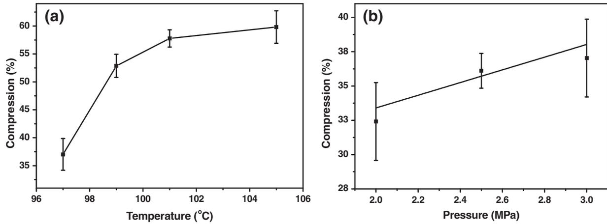
Fig. 5. Compression of the first PMMA layer at (a) different temperature with a pressure of 3 MPa and (b) different pressure with a temperature of 97 °C.
