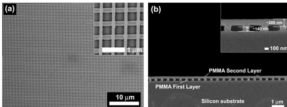
Fig. 6. SEM images of the (a) top view and (b) cross-sectional view of double-layer nanostructures. The temperature and pressure used to reverse-nanoimprint the second layer were 97 °C and 2 MPa, respectively.
