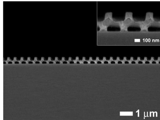
Fig. 7. SEM images of cross-sectional view of three-layer PMMA nanostructures fabricated by reverse nanoimprinting.
