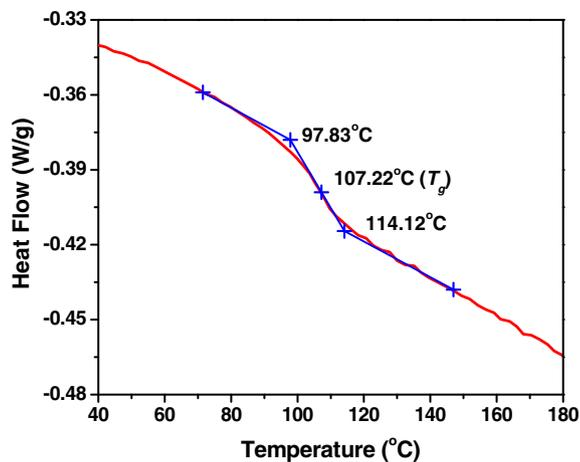
Fig. 3. DSC thermogram of PMMA (120,000 Mw).
