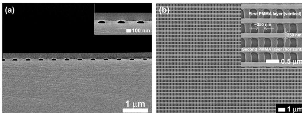
Fig. 4. SEM images of (a) cross-sectional view and (b) top view of double-layer PMMA nanostructures reverse-nanoimprinted at the  $T_g$  of PMMA (107 °C).
