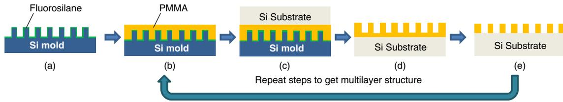
**Fig. 1.** Schematic diagram of the fabrication process for the multilayered nanostructures via reverse nanoimprinting: (a) overnight deposition of fluorosilane on silicon mold, (b) spin-coating of PMMA on fluorosilane-coated silicon mold, (c) reverse nanoimprinting process on silicon substrate, (d) removal of silicon mold from PMMA, and (e) removal of residual layer using reactive ion etching.
