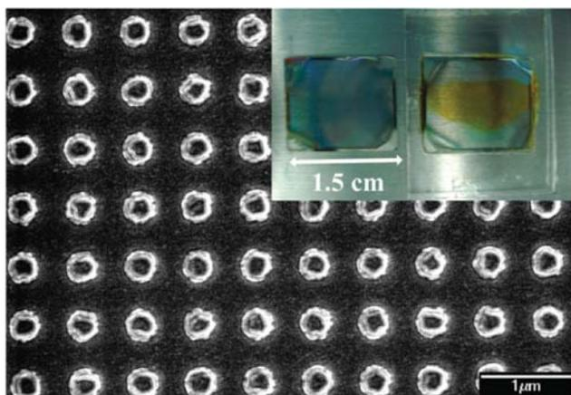
Fig. 1 Typical SEM image showing the top-view of a fabricated silver nanorod arrays. Insets are the images of the real sample before (left) and after LC (right) infiltration.
