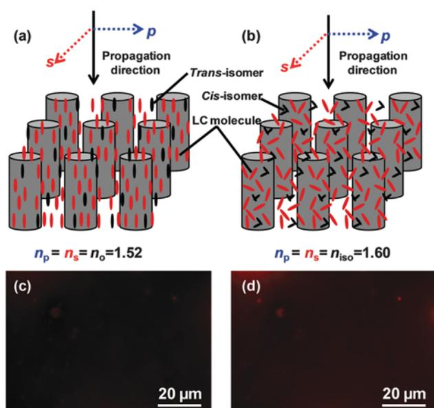
Fig. 4 The proposed model for the alignment of LC molecules inside the Ag nanorod array before (a) and after (b) the UV light pump. The observed optical images before (c) and after (d) the UV light pump between two crossed polarizers under the polarized optical microscope.
