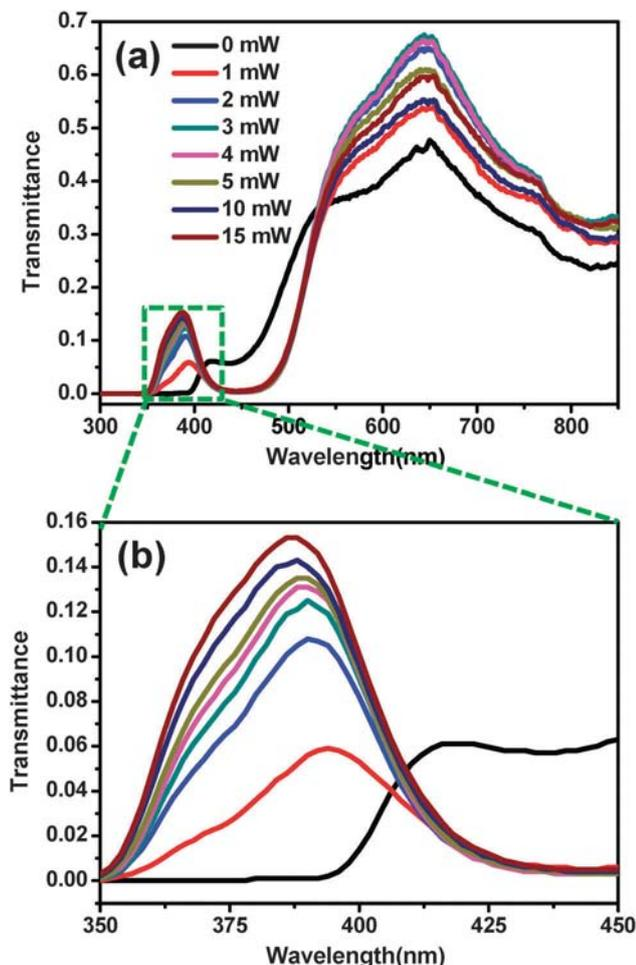
Fig. 5 (a) Effect of the pumping power on the transmission at a fixed incident angle of  $20^\circ$  and (b) magnified view of (a) in the wavelength range of 350–450 nm.
