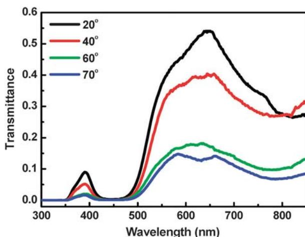
Fig. 6 Measured incident-angle-dependent transmittance at the fixed pumping power of 15 mW.
