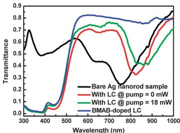
Fig. 2 Measured transmittance of the bare sample before and after LC infiltration with a UV light pump.
